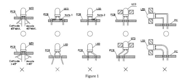
" $\circ$ " Correct mounting method, " $\times$ " Incorrect mounting method, Note 1-2:Do not route PCB Trace in the contact area between the lead frame and the PCB to prevent short-circuit.
