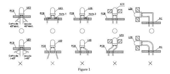
"o" Correct mounting method, "x" Incorrect mounting method, Note 1-2:Do not route PCB Trace in the contact area between the lead frame and the PCB to prevent short-circuit.
