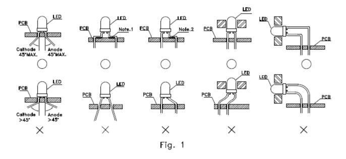
"° Correct mounting method "×" Incorrect mounting method
