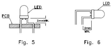
Lead forming or bending must be performed before soldering, never during or after 2. soldering.
