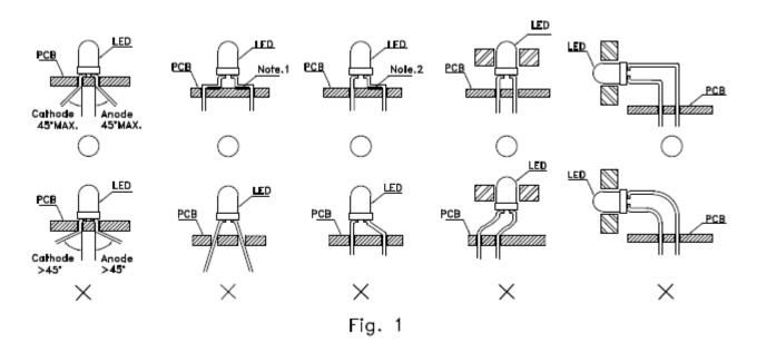
"o" Correct mounting method "x" Incorrect mounting method
