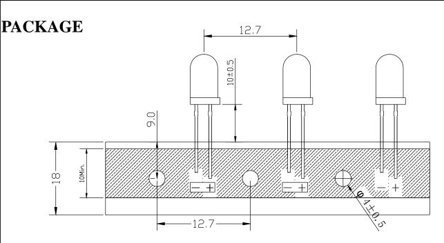
All dimensions are in millimeters. Tolerance is ±0.20mm unless otherwise noted.
